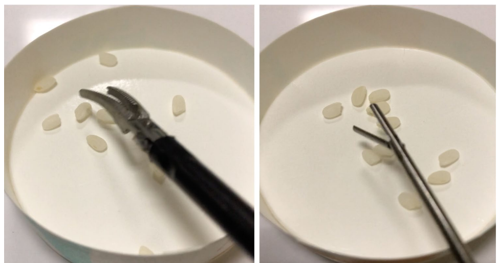
Fig. 6 A 5 mm instrument (left) obscures visualization and slows down the detection and grasping of rice grains on a small dish compared with the 2.1 mm instrument (right)
