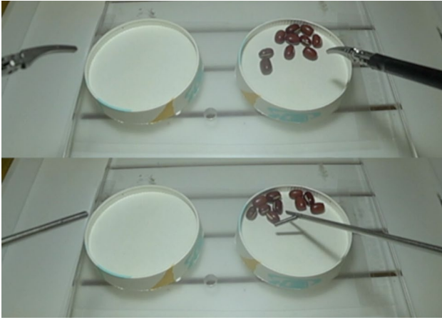
Fig. 3 Experimental setting of Task 1. Grasping and moving red beans and grains of rice
